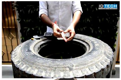
Tag developed to track finished tire, with unique identification number to prevent tire theft and cloning.
